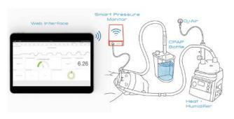
The diagram depicts a preexisting bCPAP circuit with the added smart pressure monitor. The device continuously reads the pressure of the bCPAP system and will alert nurses to abnormalities. The web interface and patient data display is accessed through an iPad or other computer.
