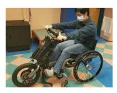
Prototype for handlebar and new control interface on a BATEC electric front-attachment, with wheelchair and user
