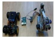
The distance detector locates the desired object, and the camera identifies and sends coordinates to the manipulator arm, which then performs the unscrewing task. The system also includes two Raspberry Pi 4 8GB microcomputers. One handles sensors and the car movement. The other handles the manipulator arm.
